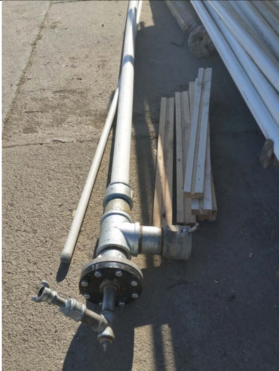
Head assembly for dual swab development tool.
